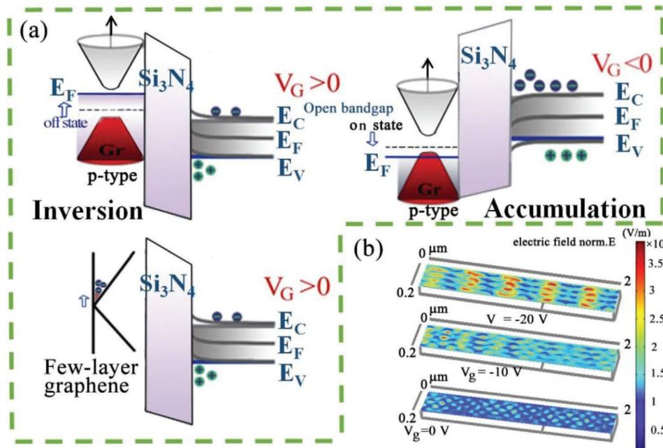
**Figure 4.** a) Schematics of device physics. b) Semiconducter-electromagnetic Multiphysics simulation for the device with different gate voltages.
