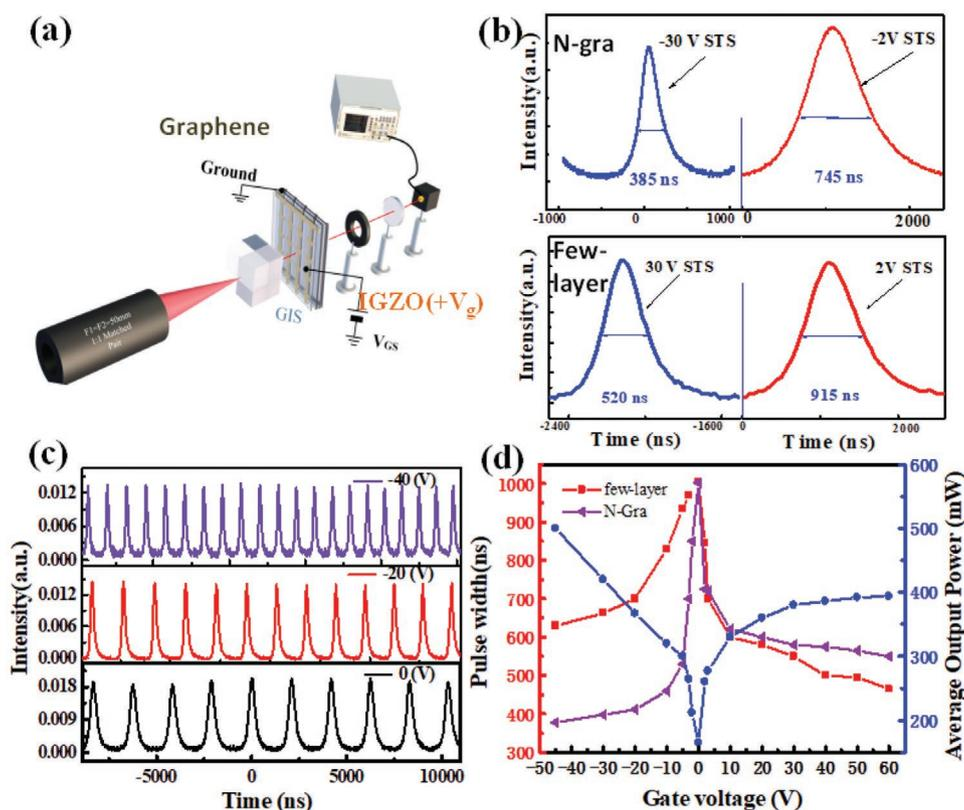
**Figure 3.** a) Experimental setup of the passively Q-switched Nd:YVO<sub>4</sub> laser. b) The enlarged waveform of the pulse for both few-layer and N-gra based devices under different applied gate voltages. c) The waveforms of the Q-switched laser at different gate biases. d) The pulse width and the average output power versus the gate voltage of few-layer graphene and N-gra based devices.
