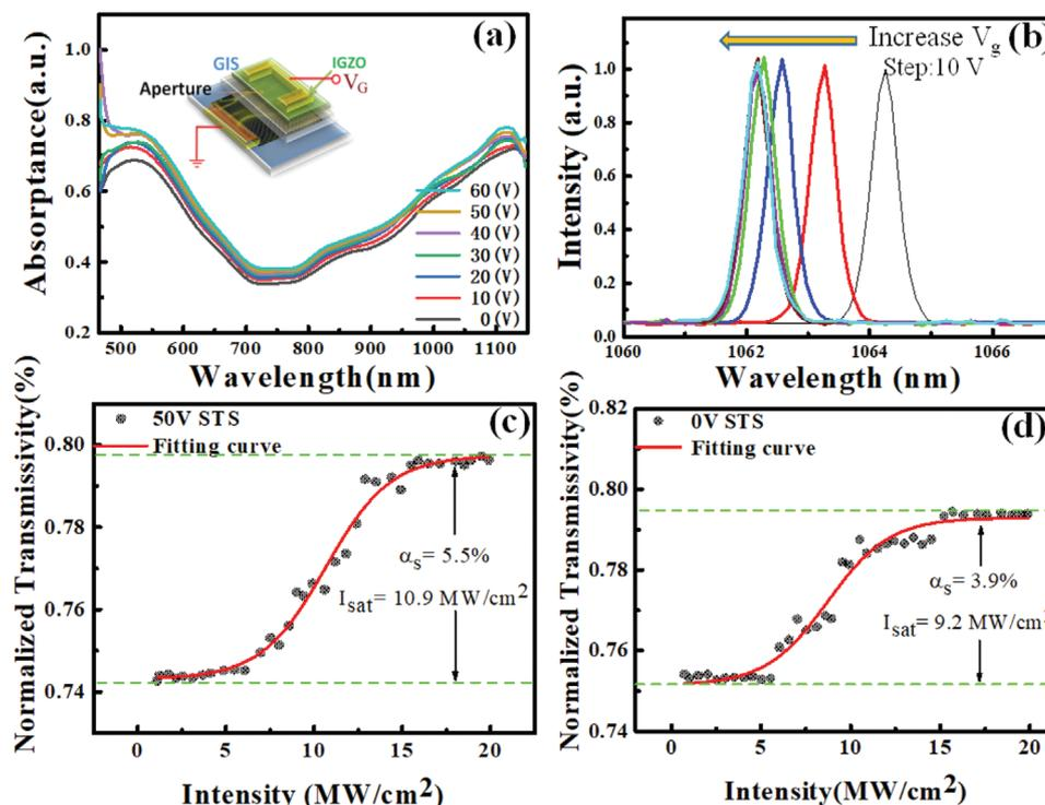
**Figure 5.** a) Optical absorption characteristic curves of GIS with N-gra SA under different gate voltages' amplitude (shown in inset images). b) Output laser spectra's blue shift under the same pump powers with increasing gate voltage amplitude from 0 to 60 V. Measuring modulation depth points of c) high and d) low voltages' amplitude of STS nanomesh-SA and their corresponding fitting curve.
