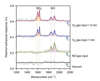
**Fig. 4** Identification of gas molecules during chemical reactions. From bottom to top: plasmon-enhanced molecular signals in a chamber filled with no gas (i.e. vacuum), 1 min and 1.5 min after  $O_2$  input. We corroborated the direct observation of the oxidation of NO to  $O_2$
