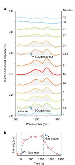
**Fig. 2** Real-time gas identification. **a** Real-time plasmon-enhanced rotational-vibrational mode response of  $SO_2$  during a full gas enter-exit cycle (data extracted from the extinction measurements reported in Supplementary Figure 10). Spectra were recorded at the times indicated on the right. **b** Kinetic plot of plasmon-enhanced  $SO_2$  signal intensity, defined as the integrated peak area in **a** as the  $SO_2$  gas enters and exits the chamber
